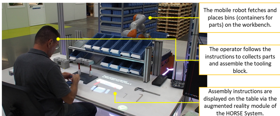
Figure 10. Photo of the TRI tool assembly process, post-intervention.
